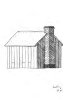
Restored lengthman's hut on the Grantham Canal, built with a brick chimney stack and reused railway sleepers. (DK-CM)
